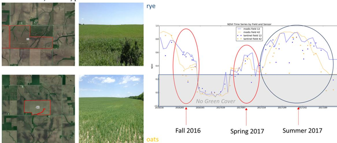
**Figure 2.** Demonstration of OpTIS estimates of winter cover. The algorithm works using a time series of Normalized Difference Vegetation Index (NDVI) as an estimate of green cover through the fall, winter, and spring.
